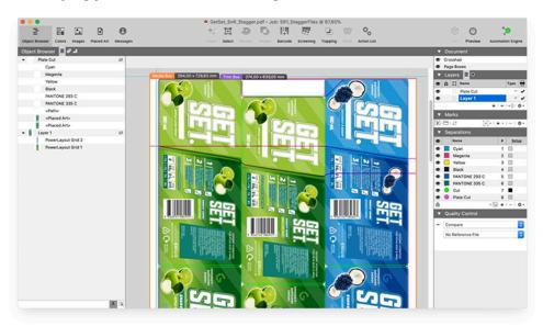
You can easily check your Plate Cutting Paths in ArtPro+ by using the **Flexo Print Preview** option in the Quality Control section. This will automatically display a continuous repetition of your layout. By enabling **Show Plate Cutting Paths** you will also see the Plate Cutting Path for the separation you are viewing.
