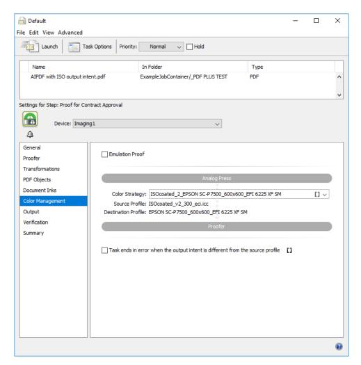
Also avoid an automatic Normalization in the background by using Dynamic Marks instead of SmartMarks! Dynamic Marks can be added in any earlier step of the workflow (for example in a PDF Action List).
