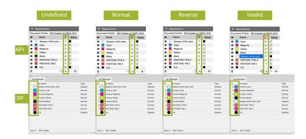
Printing Units can also be used to leave an empty patch in your mark sets, when i.e. JOB A needs to print with 7 inks, while JOB B would print with a subset of the same ink set. Using **Printing Units** you can assign the correct station number to a separation which can be reflected in marks, so I can print jobs with a (subset) of separations on the same press without setup or changeover time.
