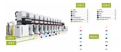
As for Automation, the **Printing Units** metadata can be used to drive workflow options such as mirroring of reverse printed jobs, naming of the output files and correctly evaluating marks.
