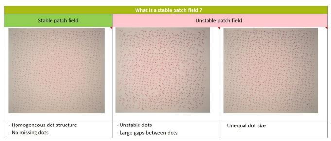
For each block, mark the stable patch that has the smallest mindot size. Please make also sure it really printed down to zero and does not stop before. At the side the position is marked with "0". If it stops printing at a higher value it means that dots got lost from the file to the print. This is not a stable situation.
