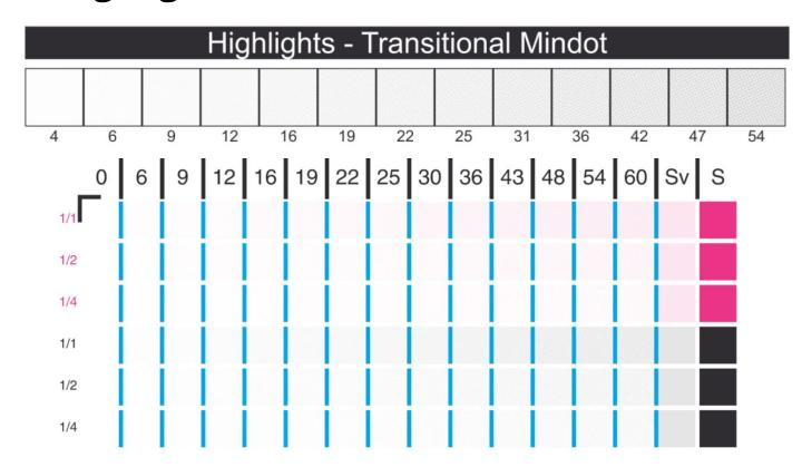
When using standard FM modulation in highlights, you must select a mindot that is large enough to print stable at the lightest tint, when dots are the furthest away from each other.
