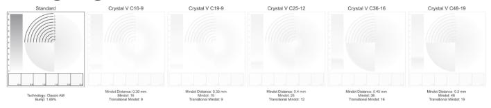
The highlights of Crystal V are set by 3 parameters: Mindot, Mindot Distance and Transitional Mindot. A range of optimal values for these parameters has been found by experience, resulting in screen presets.
