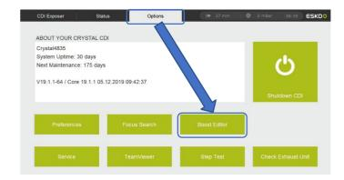
In the Boost Editor select as the Type "Plate", in Element select the used plate type in "Element" and enter the values for "Microscreen" (MCWSI) and "Groovy" (MG34). Make sure both values are entered correctly.
