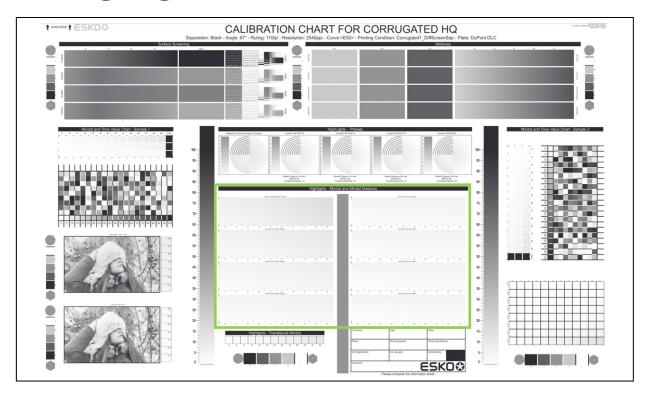
The highlight parameters can also be determined more precisely. On the Corrugated High Quality chart, below the presets, you can find an area called "Highlight Mindot and Mindot Distance", where Mindot and Mindot Distance parameters can be determined more accurately.
