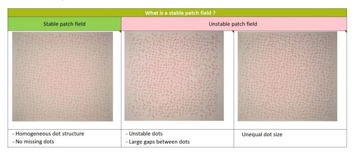
For each block, mark the stable patch that has the smallest mindot size.
