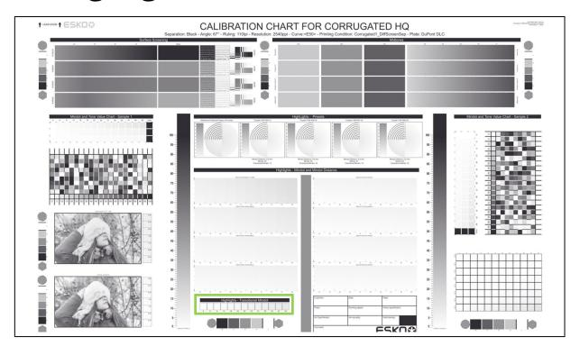
When using standard FM modulation in highlights, you must select a mindot that is large enough to print stably at the lightest tint, when dots are the furthest away from each other.
