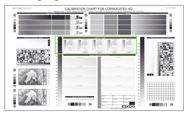
The highlights of Corrugated High Quality printing conditions are set by 3 parameters: Mindot, Mindot Distance and Transitional Mindot. A range of optimal values for these parameters has been found by experience, resulting in screen presets.
