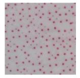
When using XPS, the print resolution in the highlights is much higher, and very small dots can also reach the printing surface of the plate. In this case you should avoid using support dots technology.
