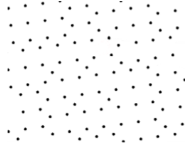
PerfectHighlights screen at 2.5% (with support dots), and print simulation (with support dots removed)
