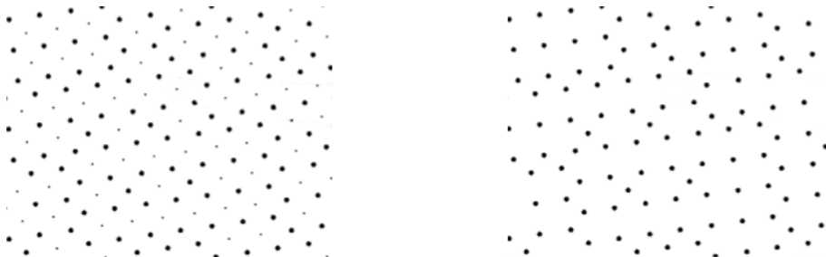
PerfectHighlights screen at 2.5% (with support dots), and print simulation (with support dots removed)
