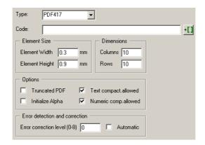
Element sizeElement Width: minimum width of the element (=bar) in mm.Element Height: height of the element (=bar) in mm.
