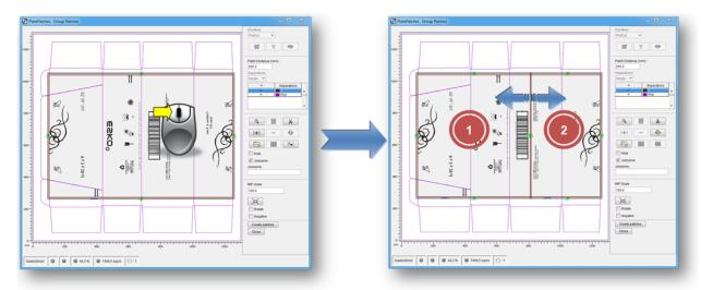
New positioning marks are added to each side apart from the seam. To manually undercut this seam, the two plate pieces overlap. In addition, a mark is added to the top and the bottom of the seam which can be used for manual cutting.
