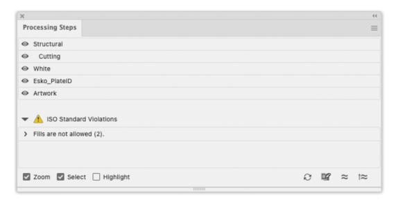
All the **Processing Steps** appear in the list, grouped per type, along with an "Artwork" entry. You can use the eye icon to make a processing step visible or invisible.
