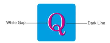
The overlap creates a dark area and the gaps cause an undesirable light area. To prevent these potential discrepancies, a trap can be implemented, causing the original colors to slightly overlap each other:
