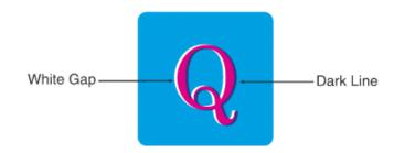
The overlap creates a dark area and the gaps cause an undesirable light area. To prevent these potential discrepancies, a trap can be added, causing the original colors to slightly overlap each other:
