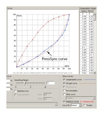
The best-fitting PressSync curve is displayed in red next to the **PressSync curve** check box. The curve is displayed dotted in red.
