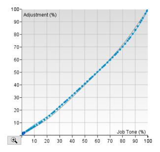
The new adjustment curve (and adjustment points) are in blue, while the previous adjustment curve (generated by the Print Control Wizard) is shown in grey.
