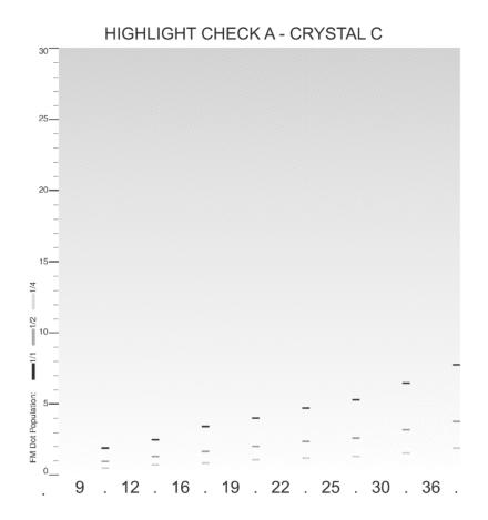
Each gradient uses a different minimum dot (the number of pixels composing the minimum dot is indicated at the bottom of the gradient).
