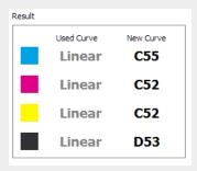
The compensation curves shown under **New Curve** in the results become the updated **Used Curve** set for the next measurement action.
