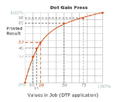
If we want to print linearly, i.e. eliminate all dot gain in the output, then we need to apply a dot gain compensation curve that is the "mirror image" of the dot gain curve for our process. This curve is shown below next to the dot gain curve for contrast.
