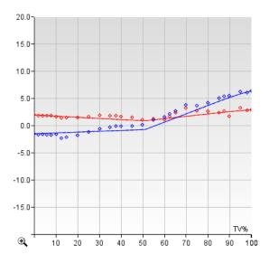
The curves obtained from this method give rise to neutral color scales in the highlights and mid tones, and to colors linearly shifting towards the measured 300% CMY patch from the feather-off tone onwards.
