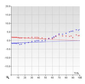
The compensation curves obtained with this method fully correct gray balance in the highlights and mid tones; in the shadows, gray tints gradually follow the natural overprint behavior of the inks.
