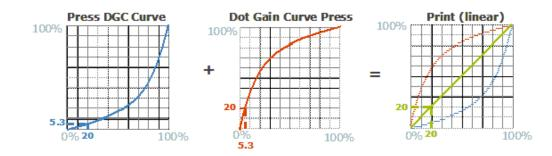
This is the principle applied during ripping and printing. Prior to screening, all intensity values are pulled down by the dot gain compensation curve (blue), leading to smaller dots on the digital film. The press "adds" its usual dot gain (red), resulting in intensity values that correspond to the original design.
