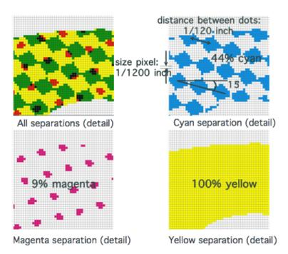
The distance between the dots in this screening raster is expressed in **lpi** (lines per inch), **lpcm** (lines per cm) or **lpmm** (lines per mm). This is called the **screen ruling**.
