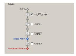
Note: Curve Pilot selects the compensation curve with the smallest lpi.
