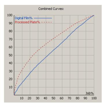
These measured data will normally form a dot gain curve that characterizes the plate processing phase of your workflow, but they can also appear in the form of a **dot loss** curve in the case of flexo printing, specifying how the plate wash-out process behaves.
