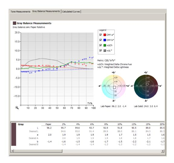
The bottom half of the **Gray Balance** tab displays measured versus desired data in a tabular format.
