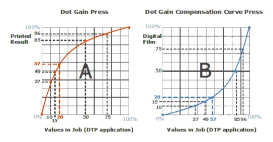
We can easily tell that data points on the dot gain compensation curve have been inverted: a tone value of 57% in the input becomes 20% in the output, while a tone value of 85% in the input becomes 50% in the output.
