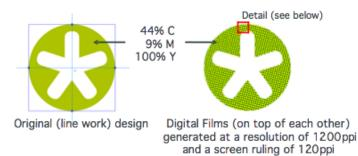
For every printing ink, the RIP application puts a raster of pixels at the resolution of the imaging device on top of the original design. To take into account the intensity of the object, the **screening** raster is added. For every pixel of the object that is lying in a dot of the screen, the pixel is set to black in the final digital film (for a positive film).
