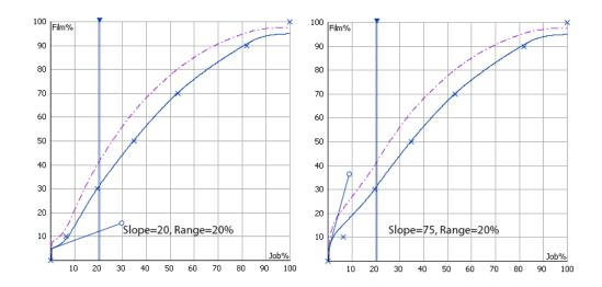
Curve Pilot lets you change the slope (and range) by dragging the slope end point with your mouse.
