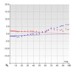
The compensation curves obtained with this method fully correct gray balance in the highlights and mid tones; in the shadows, gray tints gradually follow the natural overprint behavior of the inks.
