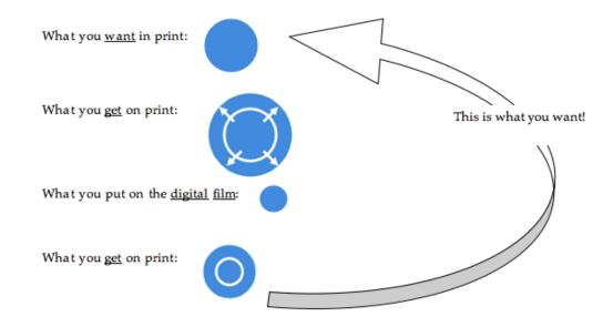
This picture explains that, in order to obtain a dot of the right size in print, a smaller dot has to be put on the digital film. In other words, applying dot gain compensation means that the original dot is **compensated** (usually reduced) to a certain extent **on the digital film**.
