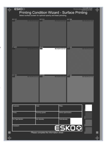
Quite often the requirement was to have a "good" white ink film, meaning that the white should appear as a clean white, covering the area below completely in a homogeneous way. Due to the limitation of the measurement equipment that is available at printer sites mainly only the opacity has been measured.
