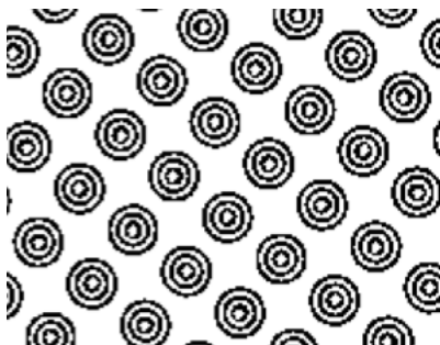
Concentric screen at 27% (with ring-shaped holes), and print simulation (with rings removed)
