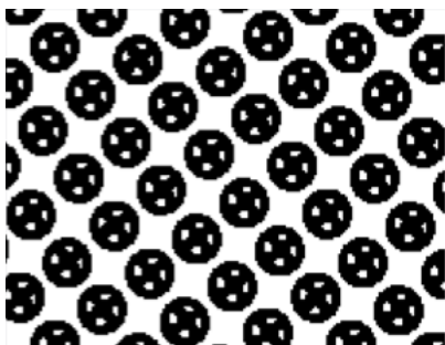
Microcell screen at 57% (with microcell holes), and print simulation (with microcell holes removed)
