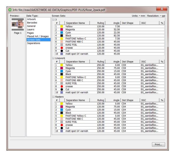
This example has 3 different sets of screens: one at ruling 120 LPI, one at ruling 250 LPI using the dot CS9 and one at 120 LPI using the dot CS4.
