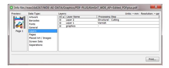
In PDF+, a layer can be of the type **Processing Step**.
