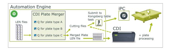
The output workflow of a *CDI Merge Queue* creates a special XML file containing the cutting instructions. When the CDI sends a signal that the (merged) plate was imaged, a workflow starts that *submits that XML file to the Kongsberg table*.
