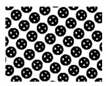
• **P+ Microcell** screens use a pattern composed of single pixels to create holes in the dots and solids. These screens are used on certain CDI devices, for example for Full HD Flexo.
