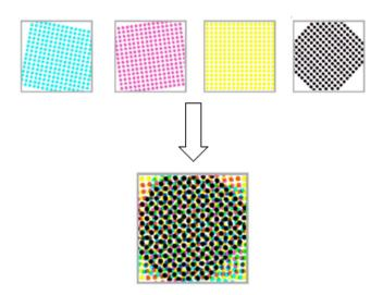
The exact screen angles used depend on the printing process:
