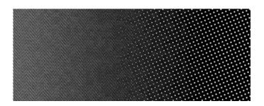
The transition between the normal screen pattern and the line pattern is smooth, leading to a smooth gradation on print between the lower density (non-groovy) and higher density areas (groovy).
