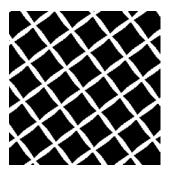
When etching the cylinder, the sharp ends are rounded off and the final result is closer to a square than the result of the standard helio dot.
