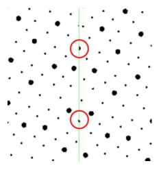
If your screen has microcells that perforate dots and solids to improve ink lay down, the microcell pattern will not repeat continuously near the seam.
