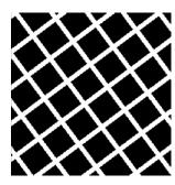
However in some circumstances the etching process smoothes out the square shape of the dots, which can cause the helio walls to break during printing (especially at the highest dot percentages), resulting in bad print quality.
