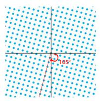
When working with such screens, you cannot place two different separations at angles that are  $90^{\circ}$  apart (if you did, the smallest registration error would cause severe *moiré*).
