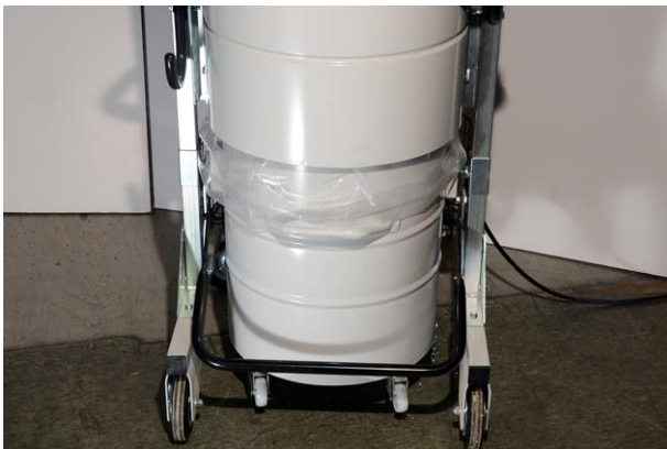
Container with plastic bag ready for operation
