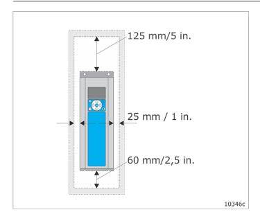
To allow for heat dissipation, ensure free space around the **Inverter**.
