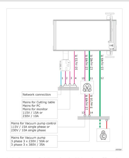
In the figure, you find alternatives for: Mains voltage / Fuse size.
