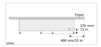
Vacuum tube to table connection, diameter 75 mm.
