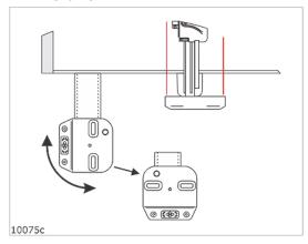
The work station top can be rotated 90°.
